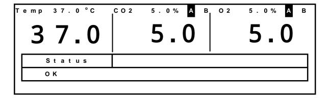
(When the line needs to be switched from cylinder A to B, press the Right Cursor Key for 3 seconds.)
